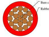
Bare copper conductor Rubber compound insulation
